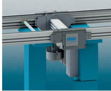
The STEIN 400 performs particularly heavy jobs. It transports heavy work-pieces weighing up to 80 kg safely and effortlessly through the production process. Despite the heavy parts, configuration and control of the system is still easy with the tried-and-trusted STEIN CONTROL Solution.
