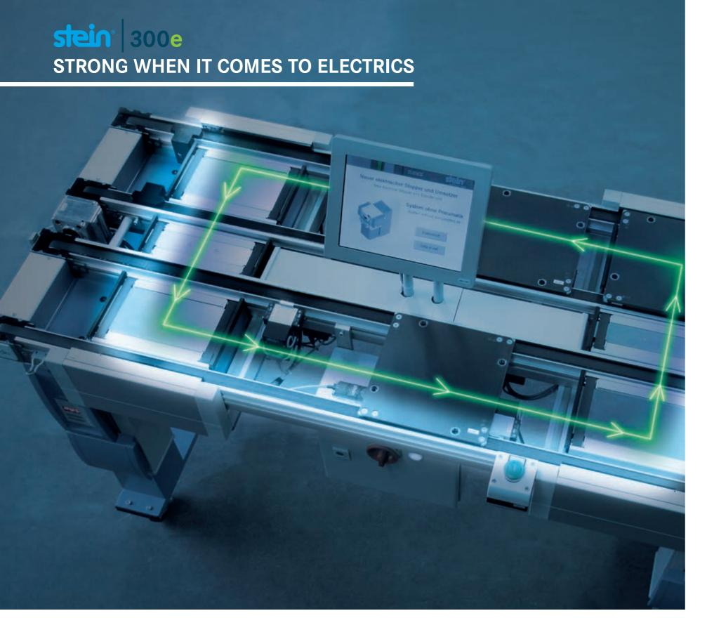
STEIN supports the trend towards electrification with the purely electric version of the 300 system - STEIN 300e. Instead of pneumatics, the stoppers, transfer units or centering devices are controlled via electric drives. This is particularly a big advantage for cleanroom applications. As a side benefit, STEIN 300e is even more energy-efficient than STEIN 300 already is.
